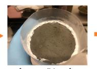
surface condition after CaCl<sub>2</sub> exposure (SME-PS)
