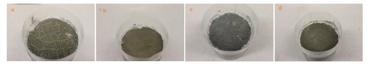
FIGURE 2 Surface condition of cement paste specimens after 14-day and 28-day exposure to 29.8% CaCl2 solution (a: control\_14d, b: SME-PS\_14d, c: control\_28d, d: SME-PS\_28d)
