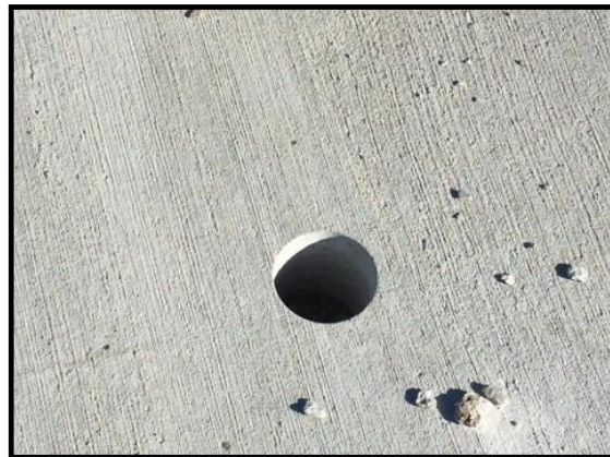
Figure 4-33: Visual Examination of a Typically Treated Pavement Fabricated from a Mixture with a w/c=0.56 , Air Volume=6.0%, and SAM=0.20 That Has Been Exposed to 10%CaCl 2
