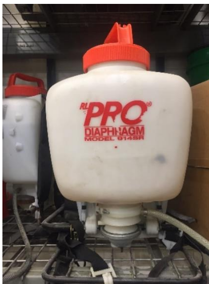
Figure 3-7: RL Pro Backpack Sprayer Used in Field Application of Deicing Salts.
