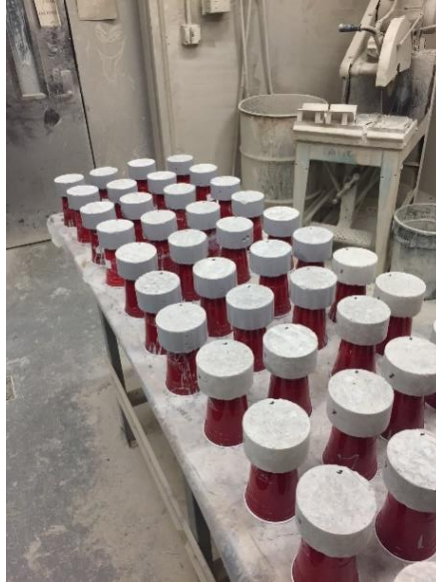
Figure 3-10: Epoxied Concrete Test Specimens
