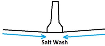
**Figure 2.15** Treatment of the median barrier at the SME-PS test section on US-231.
