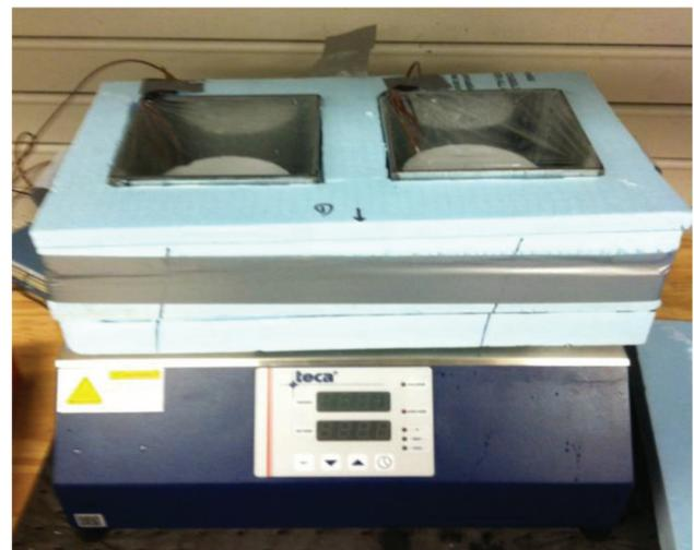
**Figure 4.1** Schematic of experimental setup for freeze-thaw absorption with chloride solution.
