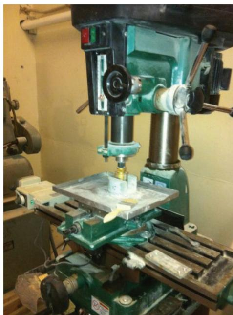
Figure 4.2 Surface grinding used to obtain powder for titration.
