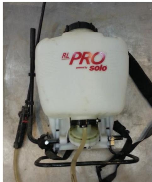
**Figure 2.12** RL Pro Flo-Master backpack sprayer used in field application of SME-PS.
