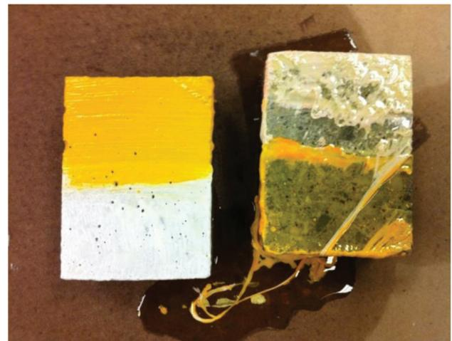
Figure 2.10 Tests of compatibility of SME-PS with INDOT road paint under normal exposure (left) and extreme exposure (right).
