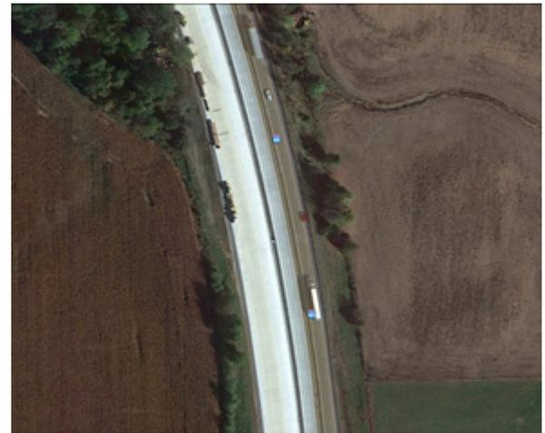
To protect the new pavement from salt and deicer, PoreShield was applied to joints on the 12-foot inside travel lane and the 10-foot end median shoulder lane. This included a centerline joint and a construction joint. Joints were spread out every 15 feet. In total, PoreShield was applied to 55,000 lineal feet of joint.
