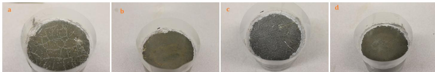
**FIGURE 2** Surface condition of cement paste specimens after 14-day and 28-day exposure to 29.8% CaCl<sub>2</sub> solution (a: control\_14d, b: SME-PS\_14d, c: control\_28d, d: SME-PS\_28d)
