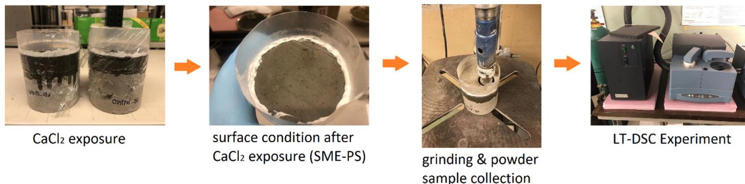
**FIGURE 1** Procedure of preparing powder samples for LT-DSC test
