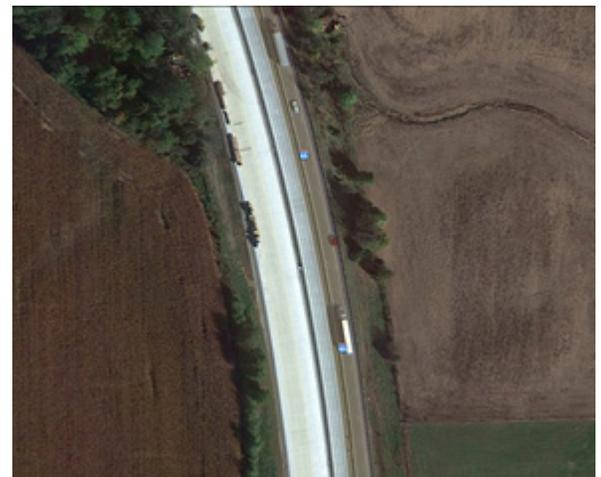
To protect the new pavement from salt and deicer, PoreShield was applied to joints on the 12-foot inside travel lane and the 10-foot end median shoulder lane. This include a center line joint and a construction joint Joints were spread out every 15 feet. In total, PoreShield was applied to 55,000 lineal feet of joint.
